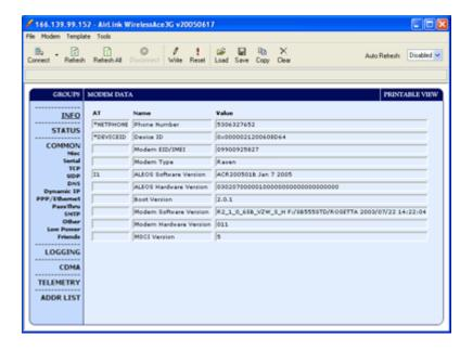
Wireless ACE can be used to monitor your Raven, view modem status, or change the configuration of your Raven. You can even save a profile and, using Wireless ACE or AceNet, apply it to another AirLink modem.
